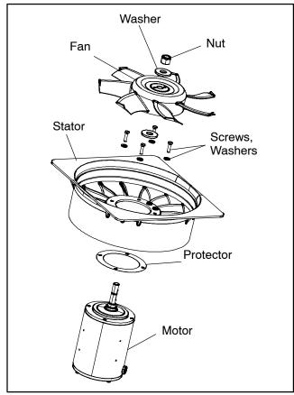
Figure 6-18 Evaporator Fan Assembly
