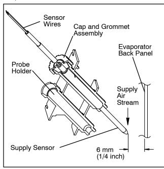
Figure 6-27 Supply Sensor Positioning
