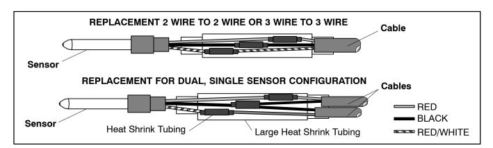
Figure 6-26 Sensor and Cable Splice
