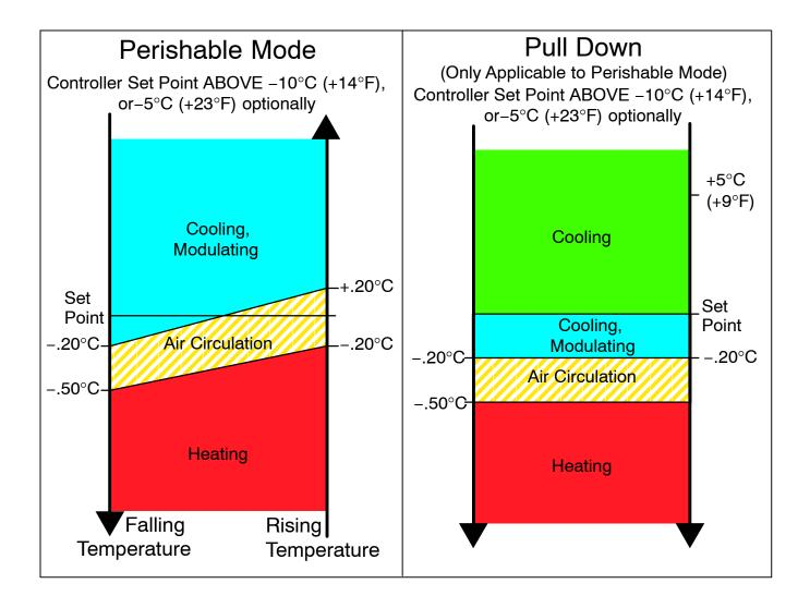
Figure 3-5 Controller Operation - Perishable Mode
