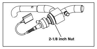
Figure 6-23 Suction Modulation Valve (SMV)
