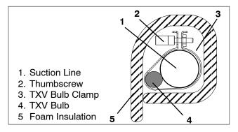
Figure 6-19 Thermostatic Expansion Valve Bulb
