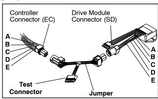
Figure 6-30 Jumper Assembly
