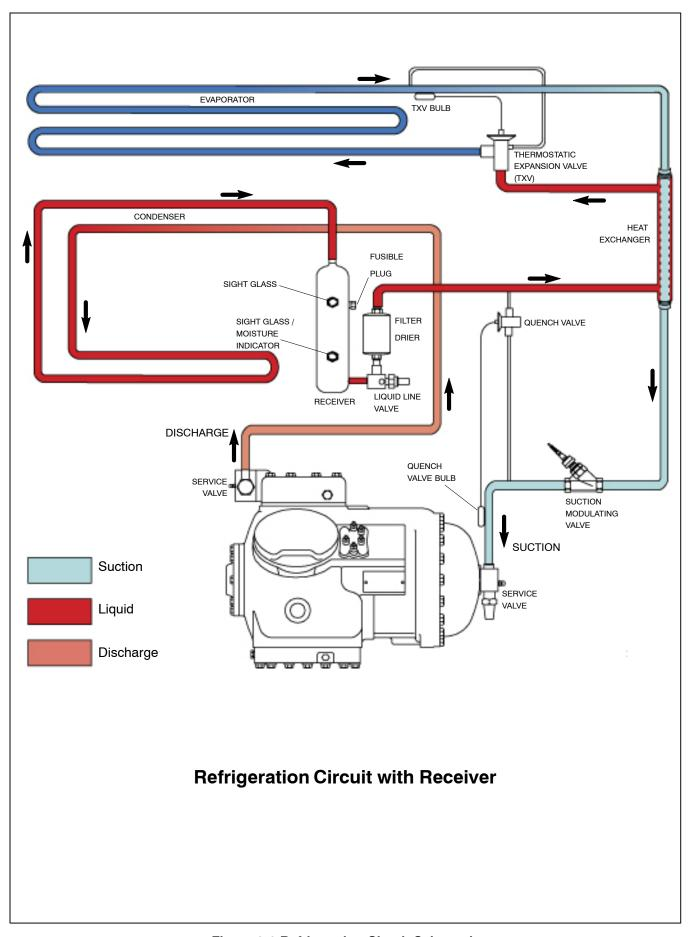
Figure 2-6 Refrigeration Circuit Schematic
