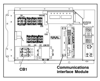
Figure 6-32 Communications Interface Installation
