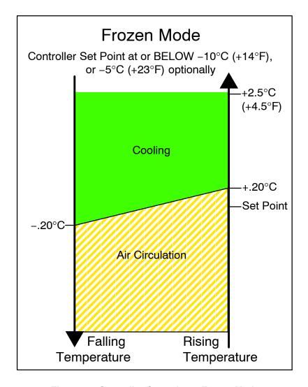
Figure 3-8 Controller Operation - Frozen Mode
