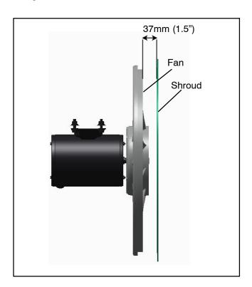
Figure 6-16 Condenser Fan Position
