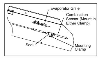
Figure 6-28 Return Sensor Positioning
