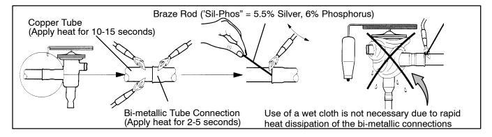
Figure 6-22 Hermetic Thermostatic Expansion Valve Brazing Procedure
