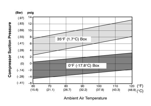
Compressor Suction Pressure Versus Ambient Air Temperature at Stable Box Temperature
